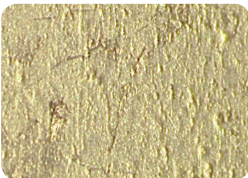
Figure 1. Blisters seen on a cold rolled 14k yellow gold sheet after annealing in a reduced atmosphere. Figure 1. Blisters seen on a cold rolled 14k yellow gold sheet after annealing in a reduced atmosphere.
