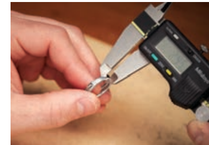
STEP 1: Measure width of shank to determine PREFORM sizing stock needed.
