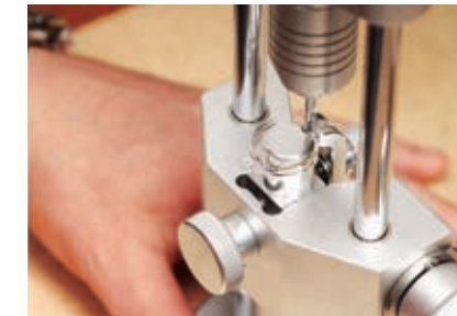
STEP 2: Select proper drill bit. Position shank. Center bottom of shank by eye. Use wheel to drive into shank.
